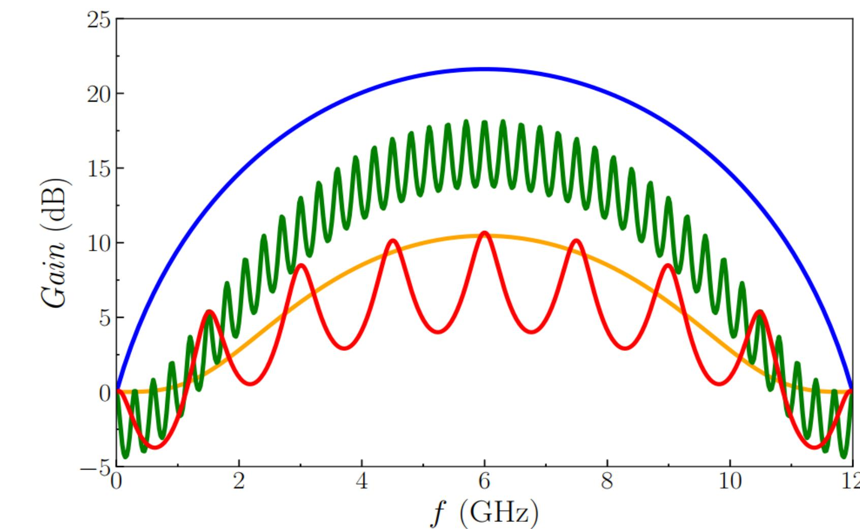
Gain profile for TWPA without reflections: orange – no phase matching, blue – perfect phase-matching. Moderate reflections ( $\Gamma = 0.6$ ) enhance both the gain and the bandwidth even without any phase-matching (green curve). Red curve is for 5-times shorter waveguide.
