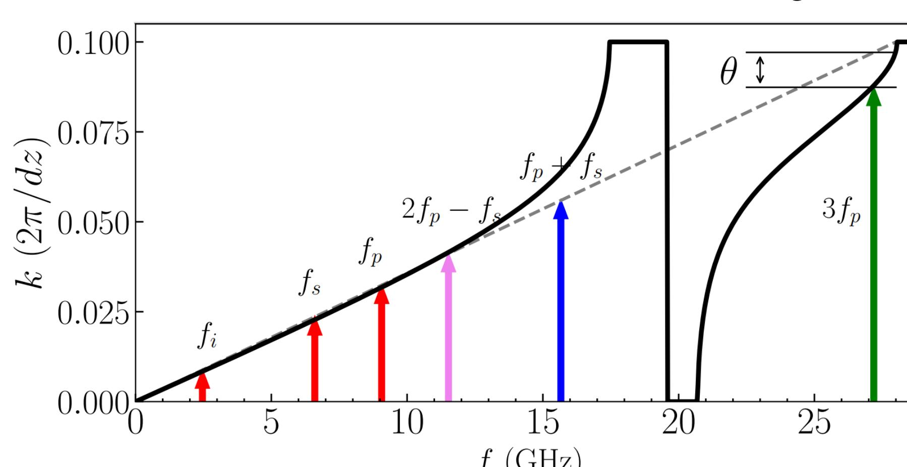
Black curve is dispersion of the PTWPA calculated by ABCD matrix method. Dashed line is the linear approximation with additional phase shift for third harmonic. Dispersion enables effective phase-matching of the THG. Indicated modes are signal, idler, pump, third harmonic and sidebands.
