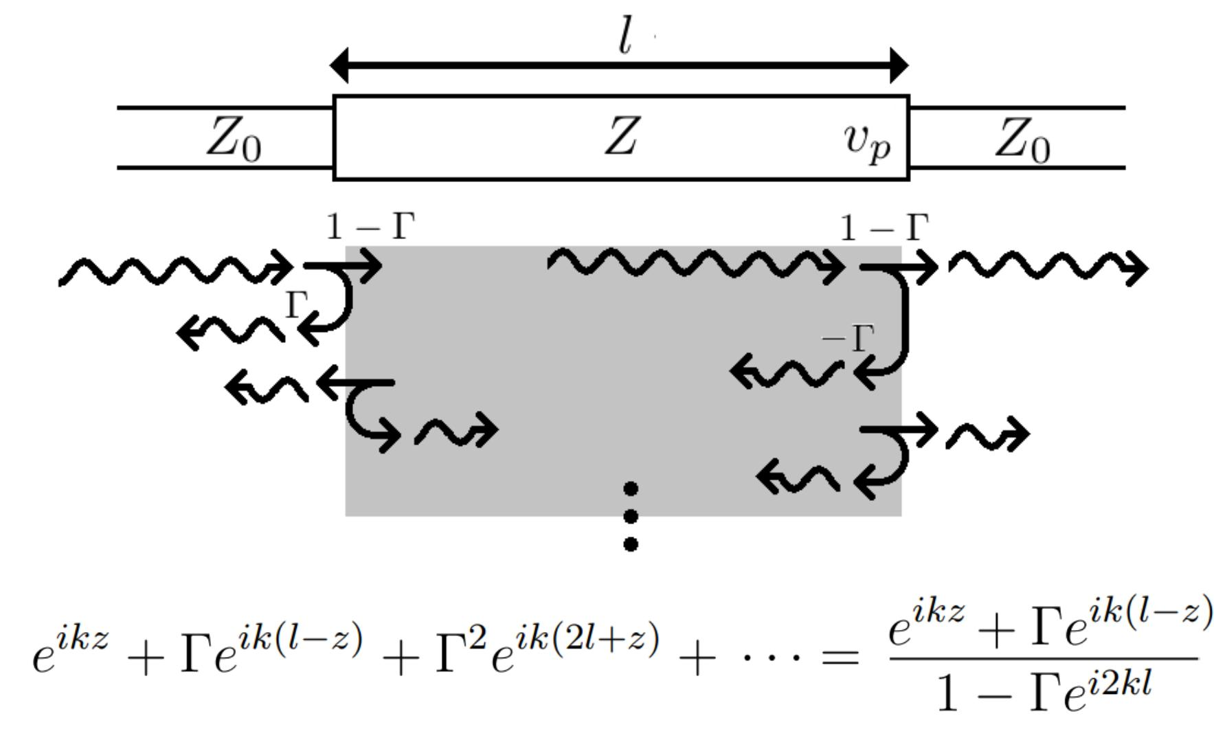
$$e^{ikz} + \Gamma e^{ik(l-z)} + \Gamma^2 e^{ik(2l+z)} + \dots = \frac{e^{ikz} + \Gamma e^{ik(l-z)}}{1 - \Gamma e^{ikl}}$$
