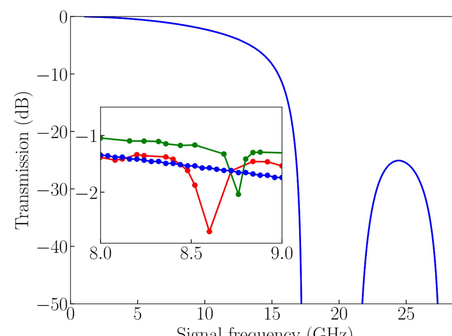
Transmission of the PTWPA probed by weak signal. The inset shows the transmission within the "sweet spot" frequency range, where amplification is enhanced, for two higher signal powers. The dip in the high-power transmission indicates efficient third-harmonic generation.
