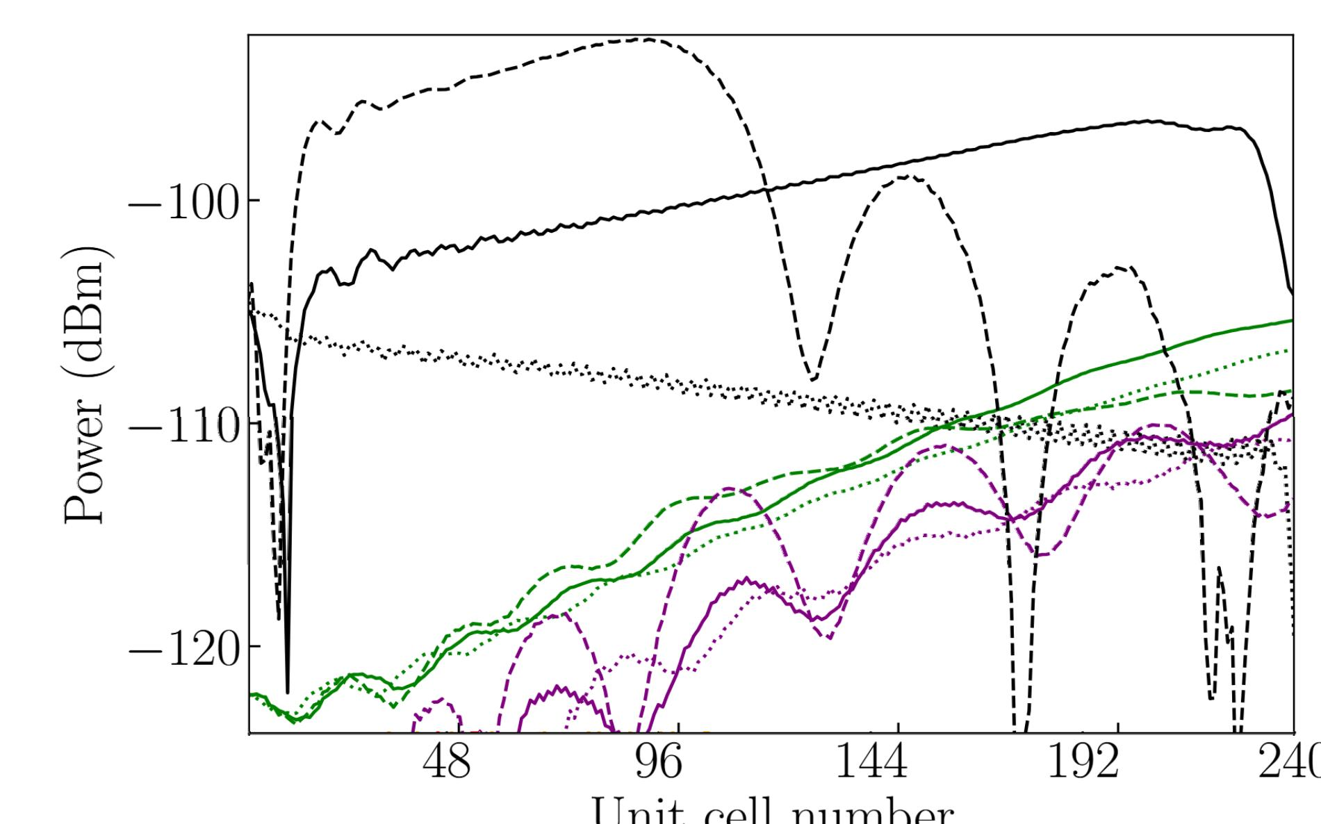
**Evolution of the respective modes:** third harmonic  $3f_p$  (black), signal  $f_s$  (green), and  $f_s + f_p$  (purple) along the PTWPA for various pump frequencies near the sweet spot, where the efficiency of third-harmonic generation can be tuned. Highly efficient THG (solid lines) is accompanied by high signal gain. This also corresponds to the widest achieved amplification bandwidth.
