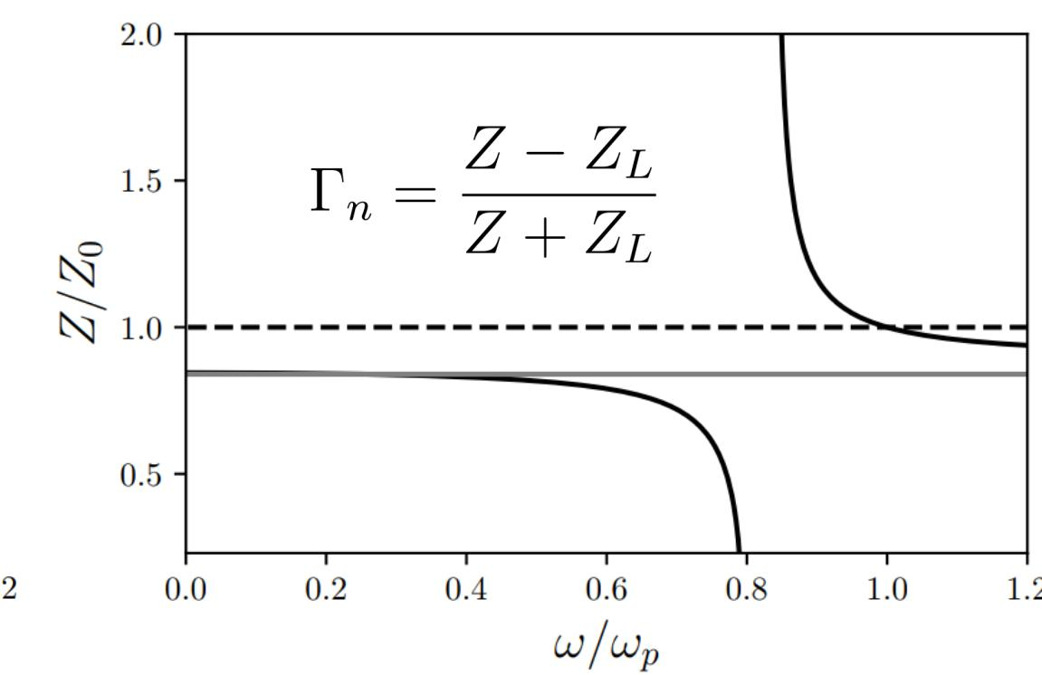
**Left:** Dispersion of resonantly loaded transmission line. Pump near the resonance introduces mismatch  $\Delta k$  satisfying phase-matching condition. However, the dispersion also enables the propagation of unwanted sidebands, such as  $\omega_p + \omega_s$ , which degrades the amplifier's gain and bandwidth. **Right:** The impedance is also modified by the resonance, leading to an impedance mismatch and causing reflections.
