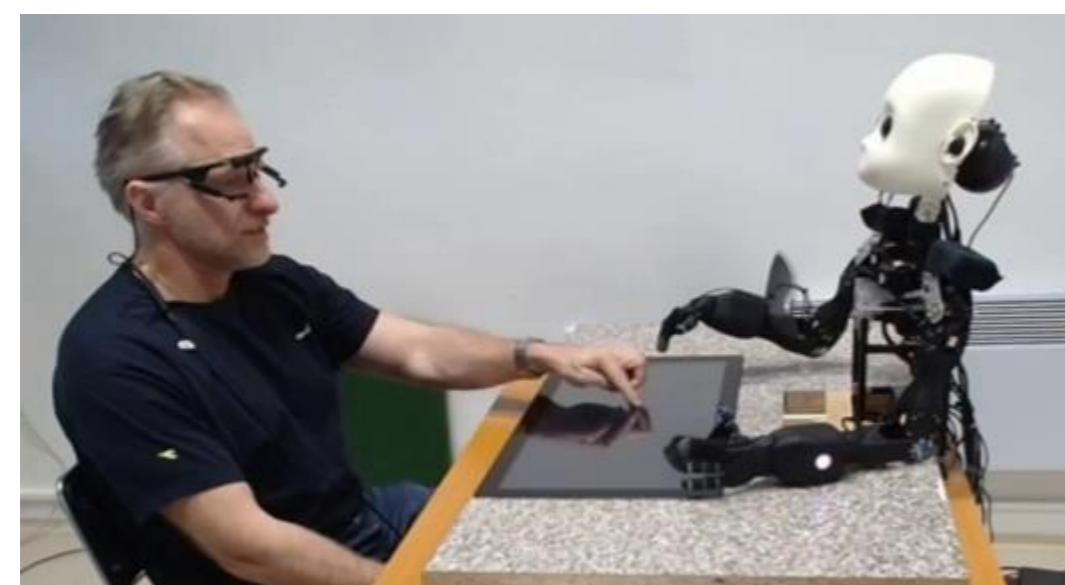
The NICO robot was programmed to point specific targets on a touchscreen, using two different modalities (the gaze and the arm movement 60 or 80% trajectory).
