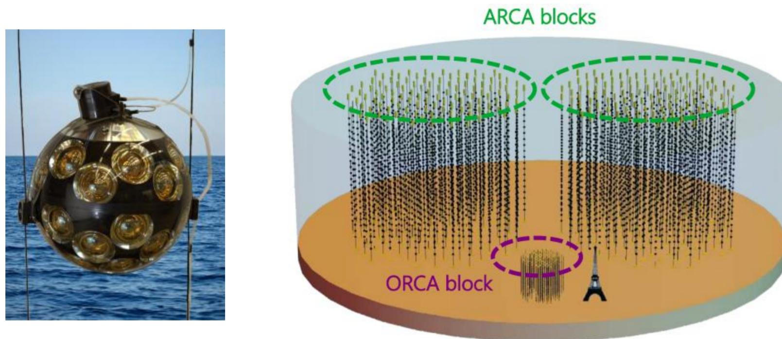
Cherenkov light that is emitted by secondary charged particles originating in neutrino interactions is detected by 31 photo-multiplier tubes inside the Digital Optical Module (DOM) that is the elementary detection unit of the telescope.
