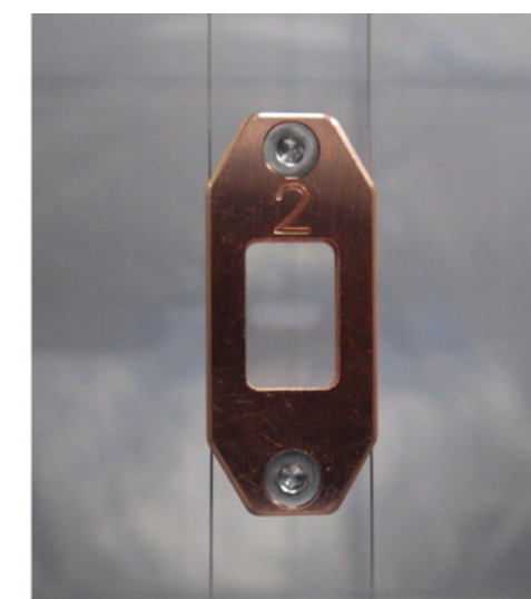
Picture of ^{207}\text{Bi} source with copper frame
